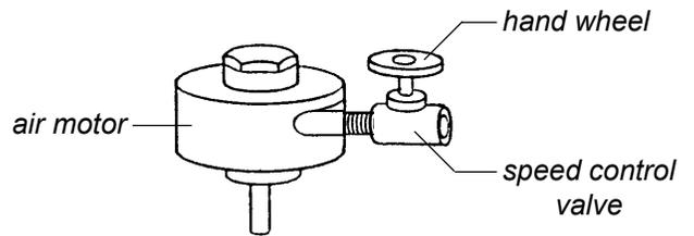
Starting torque is less than running torque and could vary depending on position at which vanes stop in relation to air intake port. Using a pressure regulator or a simple shut-off valve to obtain desired power and conserve air can regulate speed and torque.
